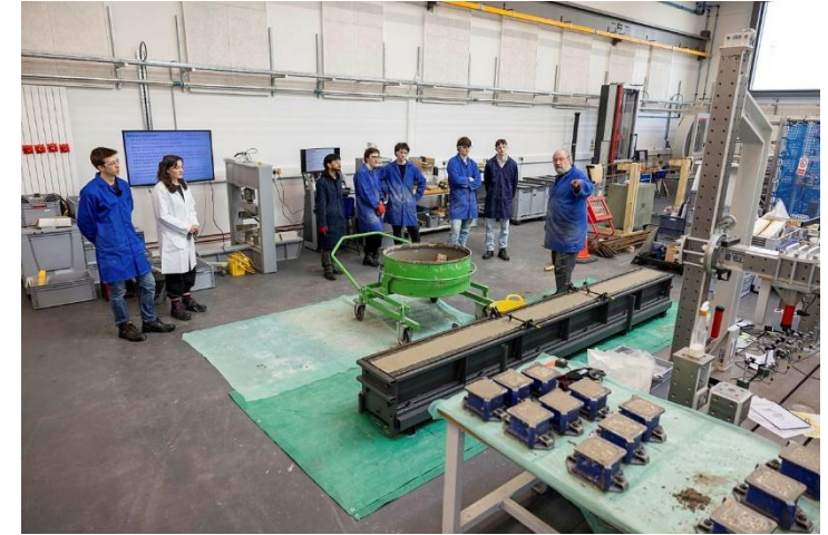
Concrete testing – cube tests, reinforced beam.
